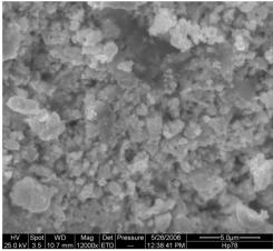
Fig. 5 SEM micrograph of copper recovered by cementation with Zn. Average particles size =  $\sim$ 500 nm.
