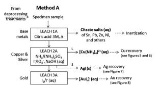
Fig. 2 Schematic diagram of the leaching steps of Method A. L, S = liquid and solid fractions.
