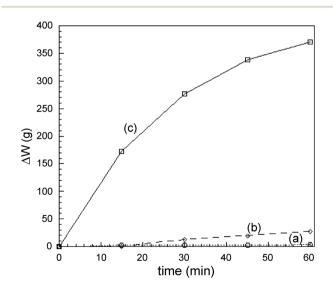
Fig. 11 Weight loss of calibrated copper wires (500 mg,  $\varnothing=0.3$  mm) in the given time (minutes) by treatment with NH $_3$ /(NH $_4$ ) $_2$ SO $_4$  (4.4 × 10 $^{-3}$  M and 6.0 × 10 $^{-4}$  M, respectively): (a) without additions (...O...); (b) with 30 mL NaOH 1.5 M/I $_2$  (5 g) solution ( $-\lozenge-$ ); and (c) 2.7 mL H $_2$ O $_2$  35% ( $-\cdot$ -) additions.
