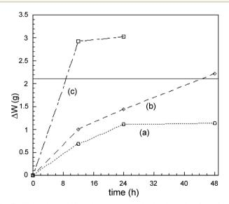
Fig. 3 Weight loss of 10 g of test specimen in the given time (hours) by treatment with citric acid 3 M at: (a) room temperature (...O...); (b) refluxing  $(-\lozenge-)$ ; (c) by  $H_2O_2$  35% addition  $(-\cdot\Box-\cdot)$ . The solid line represents the expected amount of base metals in the sample (2.1 g).
