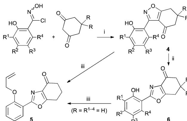
Scheme 2 Synthesis and rearrangement of 3-aryltetrahydrobenzisoxazoles **4**. Reagents: (i), NaOi-Pr, *i*-PrOH; (ii), Cs<sub>2</sub>CO<sub>3</sub>, THF reflux; (iii), H<sub>2</sub>C=CHCH<sub>2</sub>Br, Cs<sub>2</sub>CO<sub>3</sub>, THF reflux.
