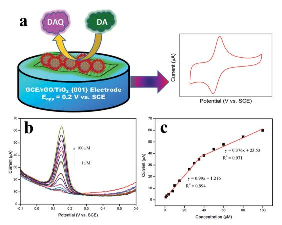
Fig. 13 (a) Mechanism for the electrocatalytic oxidation of dopamine at  $rGO/TiO_2$  {001} modified GCE. (b) DPV obtained for  $rGO/TiO_2$  {001} modified GCEs during the addition of 1, 2, 4, 8, 10, 15, 25, 30, 35, 40, 50, 60, 80, and 100  $\mu$ M DA into the 0.1 M PBS (pH = 6.5). (c) Calibration plot observed for the oxidation peak current vs. concentration of DA. Reprinted with permission from ref. 123, Copyrights (2014) Nature publishing Group.
