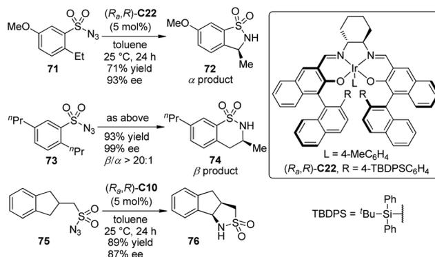
Scheme 21 The Ir-catalyzed asymmetric intramolecular C–H bond amination reactions reported by Katsuki.
