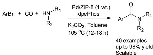
**Scheme 34** Reagents and conditions: ArBr (1 mmol, 1 equiv.), CO (4 bar), NHR<sub>1</sub>R<sub>2</sub> (1.5 equiv.), Pd/ZIF-8 (24 mg, 0.21 mol% Pd), dpePhos (1 mol%), K<sub>2</sub>CO<sub>3</sub> (1.5 equiv.), toluene (3 mL).
