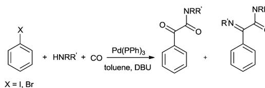
**Scheme 72** *Reagents and conditions*: aryl halide (0.05 M), amine (0.05 M or 0.1 M), DBU (0.1 M), immobilized Pd(PPh<sub>3</sub>)<sub>4</sub> (0.4 g), flow rates between 0.2 and 0.5 mL min<sup>-1</sup>, CO (40 bar), temp. 70–100 °C.
