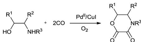
**Scheme 86** Reagents and conditions: amino alcohol (1 mmol), PdCl<sub>2</sub>(MeCN)<sub>2</sub> (0.05 mmol), CuI (0.25 mmol), acetonitrile (2 mL), CO (80 kg cm<sup>-2</sup>) and O<sub>2</sub> (5 kg cm<sup>-2</sup>), rt, time 20 h.
