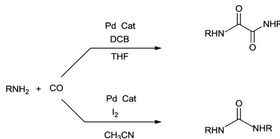
Scheme 83 Reagents and conditions: diethylamine (2.07 mL, 20.0 mmol), *trans*-[PdCl<sub>2</sub>(PPh<sub>3</sub>)<sub>2</sub>] (17.5 mg, 0.0250 mmol), THF (3 mL), 1,4-dichloro-2-butene (0.540 mL, 5.00 mmol), carbon monoxide (1 to 100 atm), rt, time 3–17 h.
