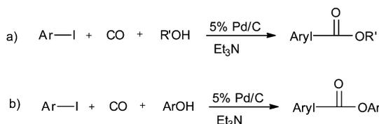
**Scheme 38** Reagents and conditions: (a) iodobenzene (2.5 mmol), 5% Pd/C (5 mg), Et<sub>3</sub>N (7.2 mmol), alcohol (4 mL), CO (0.5 MPa), temp. 130 °C, time 2 h; (b) iodobenzene (2.5 mmol), ArOH (3 mmol), 5% Pd/C (30 mg), Et<sub>3</sub>N (7.2 mmol), toluene (4 mL), CO (2.0 MPa), temp. 130 °C, time 8 h.
