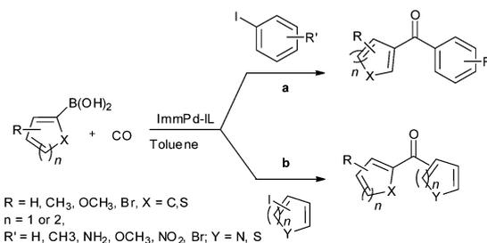
**Scheme 47** Reagents and conditions: (a) aryl iodide (1 mmol), arylboronic acid (1.2 mmol), CO pressure (1 MPa), ImmPd-IL (2 mol%), K<sub>2</sub>CO<sub>3</sub> (3 mmol), toluene (10 mL), 100 °C, 8 h; (b) heteroaryl iodide (1 mmol), heteroaryl boronic acid (1.2 mmol), CO pressure (1 MPa), ImmPd-IL (2.5 mol%), K<sub>2</sub>CO<sub>3</sub> (3 mmol), toluene (10 mL), 100 °C, 10 h.
