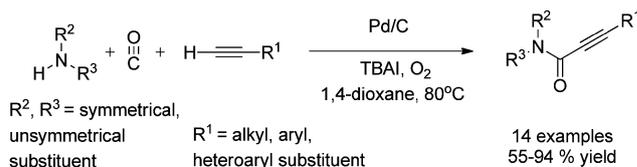
**Scheme 42** Reagents and conditions: alk-1-yne (1 mmol), secondary amine (1.5 mmol), 10% Pd/C (8 mol%), CO/O<sub>2</sub> pressure (5/1 atm), TBAI (0.90 mmol), 1,4-dioxane (10 mL), temperature 80 °C, time 14 h.
