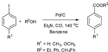
**Scheme 37** Reagents and conditions: aryl iodide (2.5 mmol), alcohol (2.5–3.0 mmol), Et<sub>3</sub>N (3 mmol), 5% Pd/C (50 mg), benzene (5 mL), carbon monoxide (1 MPa), temp. 140 °C, time 6 h.
