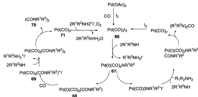
Scheme 82 Proposed reaction mechanism for the oxamide synthesis.
