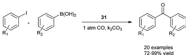
**Scheme 51** Reagents and conditions: aryl iodide (0.5 mmol), aryl boronic acid (0.6 mmol), CO (1 atm), K<sub>2</sub>CO<sub>3</sub> (1.5 mmol), **31** (1 mol%), anisole (5 mL), temp. 80 °C.
