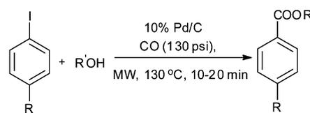
**Scheme 39** Reagents and conditions: aryl iodide (0.50 mmol), alcohol (0.50 mmol), DMF (1 mL), DBU (224 μL, 1.50 mmol), Pd/C 10% (10 mg, 0.01 mmol), CO (130 psi), temp. MW, 130 °C at 150 W, time 20 min.
