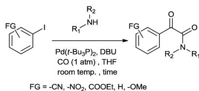
**Scheme 69** Double carbonylation of aryl iodides catalysed by a Pd(*t*-Bu<sub>3</sub>P)<sub>2</sub> catalyst.
