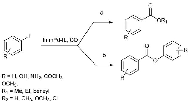
**Scheme 41** Reagents and conditions: (a) aryl iodide (1 mmol), alcohol (5 mL), ImmPd-IL (2 mol%), Et<sub>3</sub>N (3 mmol), CO pressure (0.5 MPa), temp. 80 °C, time 3 h; (b) aryl iodide (1 mmol), phenol (2 mmol), ImmPd-IL (2 mol%), Et<sub>3</sub>N (3 mmol), toluene (10 mL), CO pressure (1 MPa), temp. 100 °C, time 8 h.
