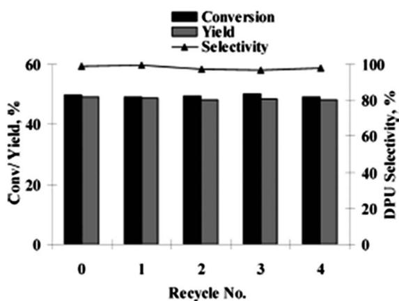
Fig. 3 Recyclability studies of the [Pd]-APTS-Y catalyst for the oxidative carbonylation of aniline. Reagents and conditions: aniline ( $0.82 \text{ kmol m}^{-3}$ ), [Pd]-APTS-Y ( $1.854 \text{ kg m}^{-3}$ ), NaI ( $1.24 \times 10^{-3} \text{ kmol m}^{-3}$ ), pressure (CO : O<sub>2</sub>) 50 psi, temp. 333 K, DMF, time 4 h.
