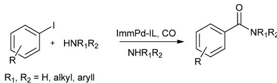
**Scheme 33** Reagents and conditions: aryl iodide (1 mmol), amine (2 mmol), ImmPd-IL (2 mol%), Et<sub>3</sub>N (3 mmol), toluene (10 mL), CO pressure (1 MPa), temp. 100 °C, time 8 h.
