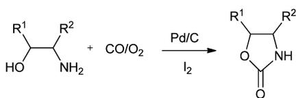
**Scheme 11** Reagents and conditions: ethanolamine (10 mmol), Pd/C (0.01 mmol), promoter (0.036 mmol), temp. 100 °C, CO (1.0 MPa), O<sub>2</sub> (0.25 MPa), DME (8 mL), time 1 h.
