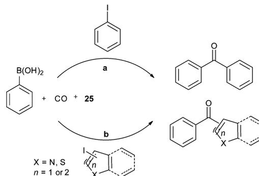
**Scheme 46** Reagents and conditions: (a) aryl iodide (1 mmol), arylboronic acid (1.2 mmol), **25** (14.5 mmol), K<sub>2</sub>CO<sub>3</sub> (3 mmol), toluene (10 mL), 100 °C, CO (100 psi), 10 h; (b) aryl iodide (1 mmol), arylboronic acid (1.2 mmol), **25** (14.5 mmol), K<sub>2</sub>CO<sub>3</sub> (3 mmol), toluene (10 mL), 100 °C, CO (100 psi), 10 h.
