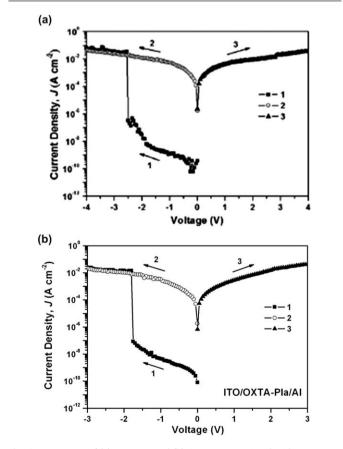
**Fig. 6** J-V curves of (a) AZTA-Pla and (b) OXTA-Pla. Reprinted with permission from ref. 18 and 20. Copyright 2010, American Chemical Society, <sup>18</sup> Wiley. <sup>20</sup>
