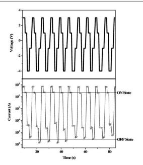
Fig. 11 The applied voltage sequence and the typical current response to WRER cycles of 3SDA-6FDA. Reprinted with permission from ref. 12. Copyright 2009, American Chemical Society
