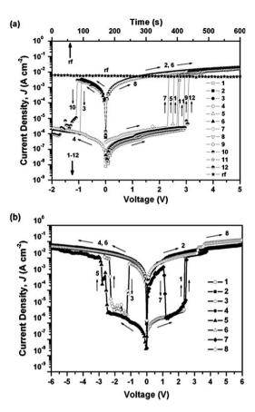
**Fig. 3** (a) The *J–V* curve of an ITO/PYTPA-PI/Al sandwich device and (b) *J–V* curve of the same device showing bi-directional electrical switching behavior. Reproduced with permission. <sup>10</sup> Copyright 2009, American Institute of Physics.
