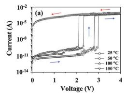
Fig. 15 /-V curves measured for the ITO/6F-HTPA PI/Al device at various temperatures under a nitrogen atmosphere. Reprinted with permission from ref. 15. Copyright 2009, American Chemical Society.
