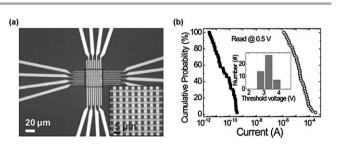
**Fig. 19** (a) An optical image of a 2 μm-scale memory device in an 8  $\times$  8 array structure. (b) A *I–V* curve of the 100 nm-scale device. Reproduced with permission.<sup>26</sup> Copyright 2011, Wiley.
