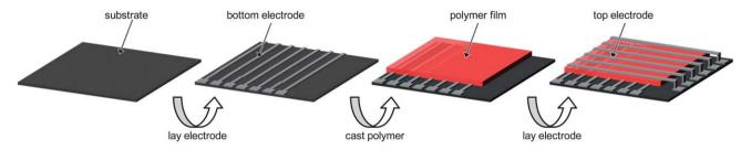
Fig. 1 A schematic diagram of the fabrication process for a polymer memory device.
