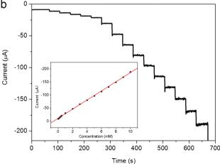
Fig. 4 (a) Cyclic voltammograms of different electrodes in  $N_2$ -saturated 0.2 M PBS at pH = 7.4 in the presence of 2 mM  $H_2O_2$  (scan rate: 50 mV s<sup>-1</sup>). (b) Typical steady-state response of the chitosan/AgNPs-G/GCE to successive injection of  $H_2O_2$  into the stirred  $N_2$ -saturated 0.2 M PBS at pH = 7.4. Inset: the corresponding calibration curve (Applied potential: -0.3 V).
