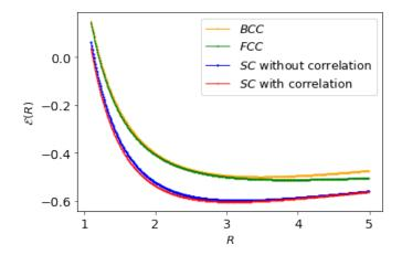
**Fig. 7** The simple formula, Eq. (18), fits neatly the energies of MH in Table 1: SC with HF (in blue) and with correlation (in red); BCC (in orange), and FCC (in green) lattice structures respectively.
