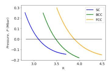
**Fig.** 8 We plot the pressure P in Mbar for MH in SC (in blue), BCC (in green), and FCC (in orange) lattices as a function of R.
