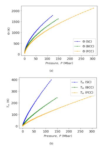
**Fig. 9** We plot the Debye temperatures  $\Theta$  (top panel) and melting points  $T_m$  (bottom panel) of MH in SC, BCC, and FCC lattice structure with the correlation with respect to the pressure, *P*.
