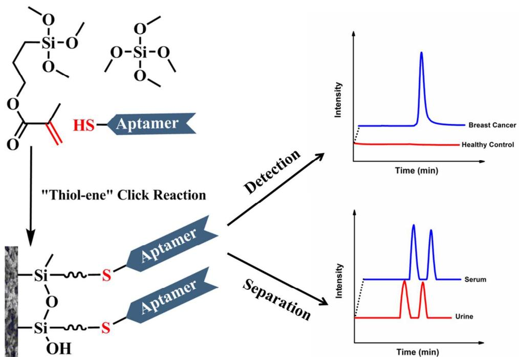
Preparation of aptamer-based organic-silica hybrid monolithic capillary column by "thiol-ene" click chemistry for detection of enantiomers of chemotherapeutic anthracyclines.
