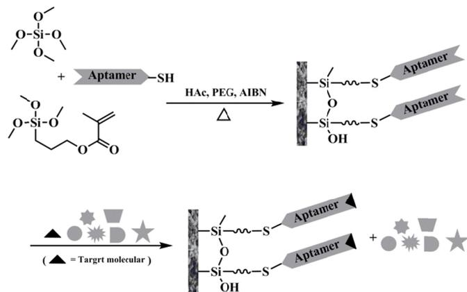
**Figure 1.** Schematic procedure for the preparation of aptamer-based organic-silica hybrid monolithic capillary column by sol-gel method combined with “thiol-ene” click reaction.
