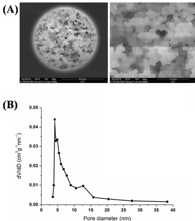
Figure 3. (A) Scanning electron microscope images of aptamer-based organic-silica hybrid monolithic capillary column. Left: 1300 $\times$ wide-view. Right: 5000 $\times$ close-up-view. (B) Mesoporous distribution of the aptamer-based monolithic column.
