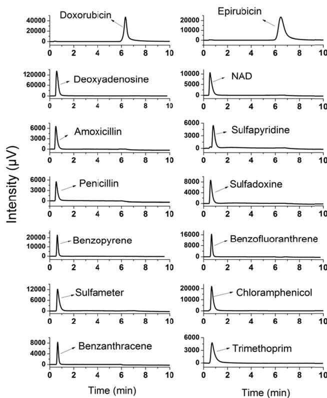
**Figure 5.** Evaluation of the specificity of the aptamer-based organic-silica hybrid monolithic capillary column. Monolithic capillary column: 10 cm-long, 75  $\mu\text{m}$  i.d.  $\times$  360  $\mu\text{m}$  o.d.; flow rate, 0.5 mL/min; inject volume, 20  $\mu\text{L}$ ; splitting ratio, 1/500; detection wavelength, 254 nm.
