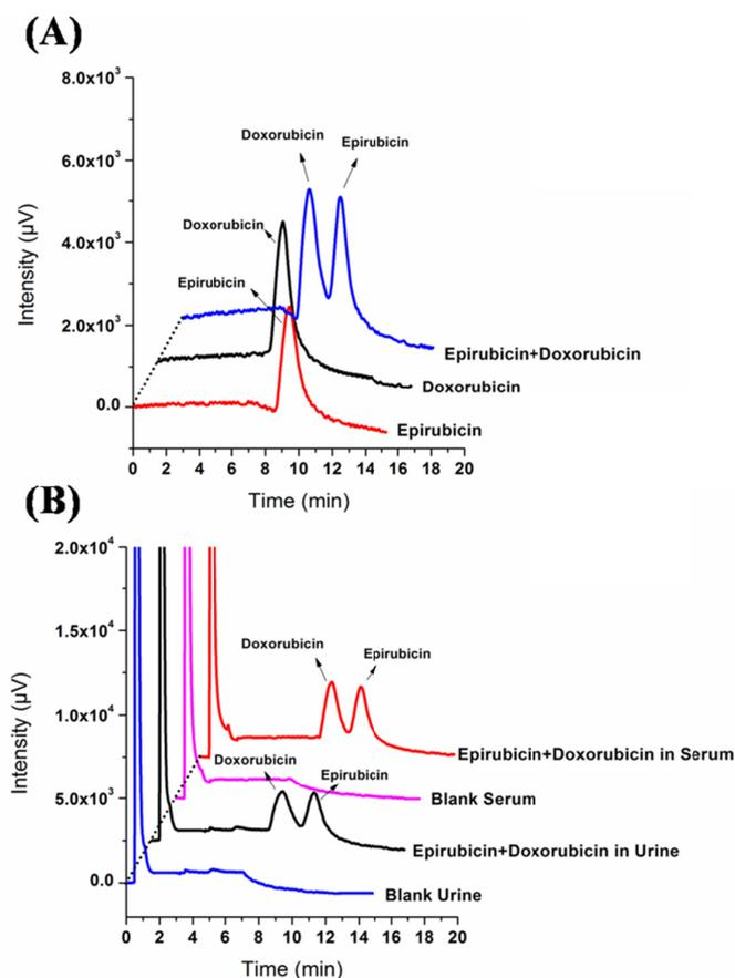
**Figure 7.** Separation of the enantiomers of doxorubicin and epirubicin spiked in water (A) or spiked in serum and urine (B). Monolithic capillary column: 10 cm-long, 75  $\mu\text{m}$  i.d.  $\times$  360  $\mu\text{m}$  o.d.; flow rate, 0.5 mL/min; inject volume, 20  $\mu\text{L}$ ; splitting ratio, 1/500; detection wavelength, 254 nm.
