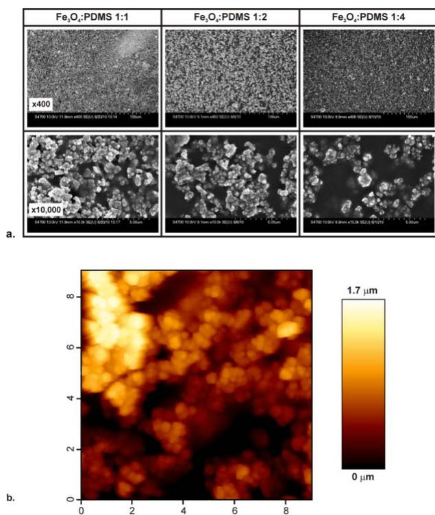
**Figure 2.** SEM and AFM characterization of magnetite-PDMS substrates. (a) SEM images taken at x400 and x10,000 magnification of three substrates with different magnetite:PDMS ratios. (b) A typical AFM image of 1:1 magnetite-PDMS substrate.
