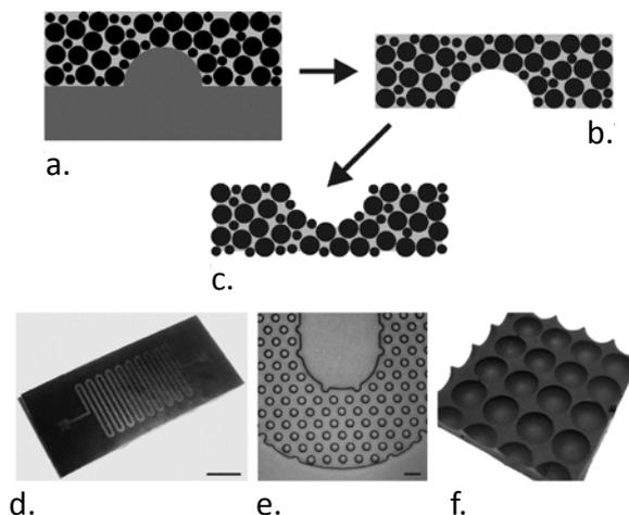
**Figure 1.** Fabrication of magnetite-PDMS structures. (a-c) The fabrication process. PDMS prepolymer is mixed with magnetite particles and cast over a suitable mold (a). After curing, the magnetite-PDMS is peeled off (b) and the surface PDMS etched back (c) to expose the embedded magnetite particles. (d and e) show an example of a microfluidic channel (50  $\mu\text{m}$  deep) fabricated from magnetite-PDMS (1:1 particle:PDMS ratio). The mold used for casting this channel was fabricated as
