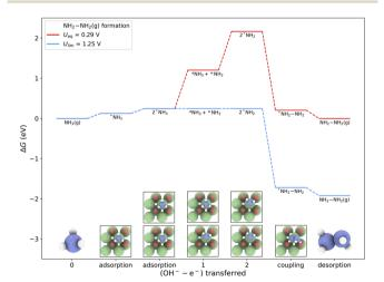
Fig. 11 Free energy diagram of hydrazine (N<sub>2</sub>H<sub>4</sub>) formed through the coupling between two \*NH2 intermediates. This mechanism avoids the deprotonation steps to form \*NH and \*N. Energy of desorption is calculated to be -0.25 eV. Equilibrium (red trace) and limiting (blue trace) potentials are calculated using the computational hydrogen electrode at pH 11.
