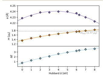
Fig. 5 Lattice constant (a), magnetic moment (m), and band gap ( $\Delta E$ ) calculated for the NiO surface using a range of Hubbard U values from 0–8. The Hubbard U value was chosen based on the closest match to experimental values for the magnetic moment. However, the calculated band gap and lattice parameter also agree with experimental values of NiO.
