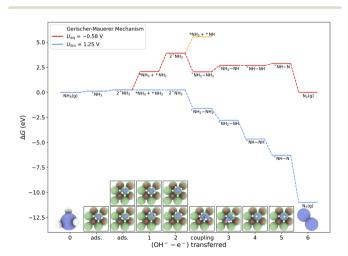
Fig. 10 Free energy diagram of N<sub>2</sub>(g) formation from AOR coupling through two \*NH<sub>2</sub> intermediates (Gerischer–Mauerer mechanism).<sup>38</sup> Equilibrium (red trace) and limiting (blue trace) potentials are calculated using the computational hydrogen electrode at pH 11.
