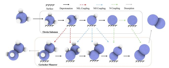
Fig. 1 AOR mechanisms toward N<sub>2</sub> and N<sub>2</sub>H<sub>4</sub> formation. Blue and white spheres are nitrogen and hydrogen atoms, respectively. The Oswin-Salomon mechanism and the Gerischer-Mauerer mechanism are outlined by a black and orange box, respectively.
