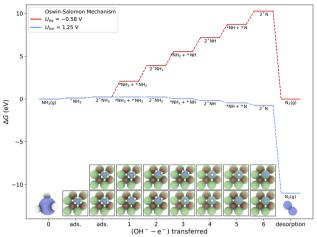
Fig. 9 Free energy diagram of N<sub>2</sub>(g) formation from AOR coupling through two \*N intermediates (Oswin-Salomon mechanism).37 Equilibrium (red trace) and limiting (blue trace) potentials are calculated using the computational hydrogen electrode at pH 11.
