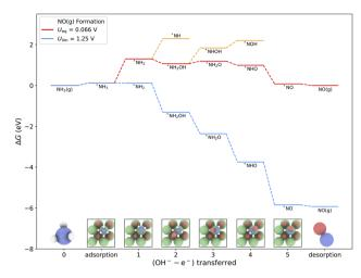
Fig. 12 Free energy diagram of NO(g) formation. This pathway includes the same initial steps of nitrite and nitrate formation, proceeding through \*NH2OH. Steps towards \*NH and \*NHOH are bypassed as their energies are less favoured. The desorption energy for NO(g) was calculated to be -0.080 eV. The equilibrium (red trace) and limiting (blue trace) potentials were calculated using the computational hydrogen electrode at pH 11.
