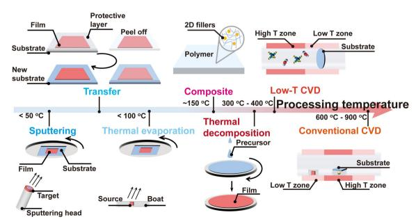
Fig. 3 Comparison of different preparation methods for 2D materials with a focus on the processing temperature.
