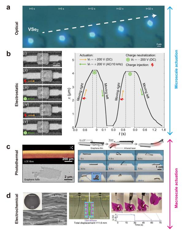
Fig. 4 Various actuation mechanisms for 2D materials. (a) Optical actuation. Reproduced with permission.<sup>68</sup> Copyright 2023, Springer Nature. (b) Electrostatic actuation. Reproduced with permission.<sup>69</sup> Copyright 2025, Springer Nature. (c) Photothermal actuation. Reproduced with permission.<sup>11</sup> Copyright 2025, Springer Nature. (d) Electrochemical actuation. Reproduced with permission.<sup>77</sup> Copyright 2024, John Wiley and Sons.
