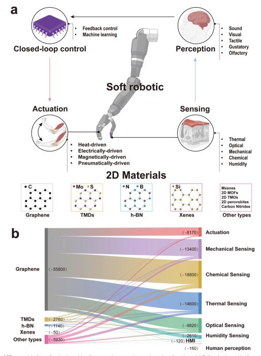
Fig. 1 Overview of 2D materials for soft robotics with a focus on the actuation and sensing directions. (a) Soft robotic and its four core units: actuation, sensing, perception (decision-maker) and control part. Created using BioRender: https://BioRender.com. (b) Sankey diagram visualizing the use of different 2D materials with various applications. Each vertical bar represents the number of publications per field. Data: Web of Science till the end of January 2025
