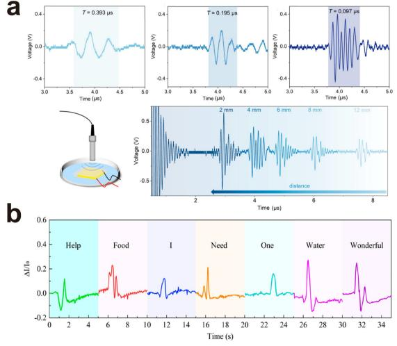
Fig. 9 2D materials for sound perception. (a) Ultrasound detection via a 2D perovskite-based acoustic sensor. Reproduced with permission.<sup>210</sup> Copyright 2023, American Chemical Society. (b) Voice recognition using a piezoelectric acoustic sensor, coupled with machine learning. Reproduced with permission.<sup>216</sup> Copyright 2022, American Chemical Society
