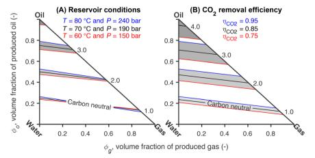
Fig. 4 Sensitivity of the  $\xi$  isolines to: (A) reservoir conditions, namely T and P within the ranges of 60–80 °C and 150 bar to 240 bar, and (B) CO<sub>2</sub> removal efficiency of DAC and EOR between 0.75 and 0.95. Black lines are the central values; blue and red lines are the best and worst climate impact scenarios within the ranges.
