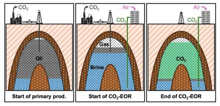
Fig. 2 Schematic representation of an oil and gas reservoir at the start of primary production, at the start of CO<sub>2</sub>-EOR (*i.e.*, after water flooding during secondary production), and at the end of CO<sub>2</sub>-EOR.
