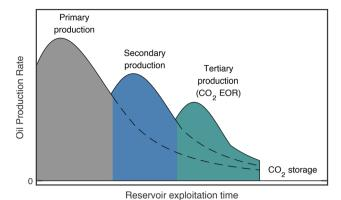
Fig. 1 Qualitative illustration of the oil production phases. Water is injected during secondary production, while CO2 is injected during tertiary production, i.e., CO2-EOR, and for storage in the depleted reservoir. Dashed lines represent oil production without transitioning to subsequent production phases.
