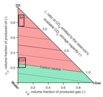
Fig. 3 Ternary diagram of the volume fraction of produced fluids (oil, gas, and water). The lines represent isolines of  $\xi$ . The squares illustrate typical phase distributions during EOR only (labelled 'EOR') and over the entire reservoir lifetime, including prior exploitation phases ('All').
