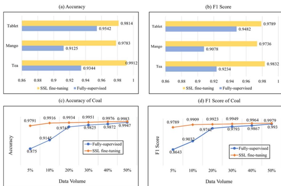
Fig. 5 Figures (a) and (b) illustrate the classification accuracies and F_1 score of tea, mango and tablet utilizing supervised learning and self-supervised learning methodologies. Figures (c) and (d) present the classification accuracies and F_1 score across 12 categories in Coal, also employing supervised learning and self-supervised learning.
