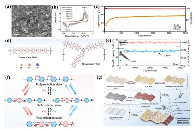
Fig. 8 (a) SEM image of PANI. (b) CV plot at different scan rates. (c) Capacity and CE vs. cycle number at 0.2 A g<sup>-1.99</sup> (d) schematic of conventional PANI and C-PANI. (e) GCD cycling performance of PANI vs. C-PANI in aqueous electrolyte. (f) Schematic of the charge storage mechanism via C-PANI. (g) Synthesis schematic of FREBs. 108
