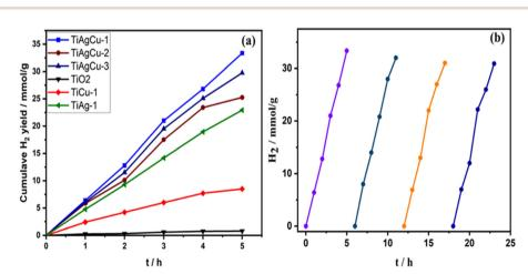
Fig. 7 (a) Time on stream dependence of solar hydrogen production of the mesoporous TiO2, TiAg-1, TiCu-1 and TiAgCu nanocomposites (in thin film form) from solar hydrogen evolution. (b) Solar hydrogen production as a function of time with repeated cycles of operation for TiAgCu-1 in direct sunlight.
