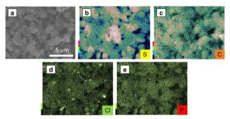
Fig. 7 (a) The SEM images of SE-S-C under an Ar atmosphere, and the EDS mapping of (b) S, (c) C, (d) Cl, and (e) P.
