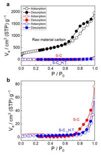
Fig. 3 (a) The N<sub>2</sub> adsorption/desorption isotherms of the raw material carbon, S-C and S-C\_H.T. (b) The enlarged N2 adsorption/desorption
