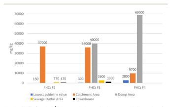
Fig. 6 PHCs (mg kg $^{-1}$ ) detected above the lowest guideline value for F2, F3 and F4 (150, 300, and 2800, respectively) at four areas. The highest value in each area of the four is shown in the figure.
