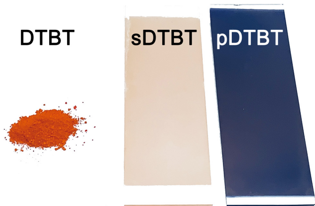
Fig. 1 Optical images of the DTBT monomer powder (orange), the sublimed sDTBT (0) coating (orange) and oCVD pDTBT (13) coating (blue) prepared from DTBT on glass substrates.
