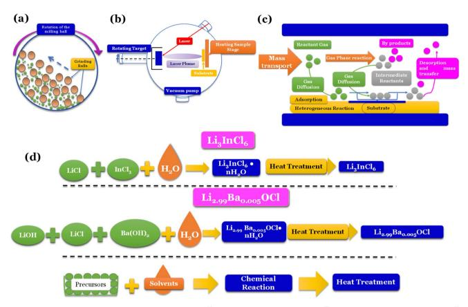
Fig. 5 Synthesis methods: (a) high energy density ball milling;<sup>76</sup> (b) pulsed laser deposition (PLD);<sup>77</sup> (c) chemical vapor deposition (CVD);<sup>78</sup> (d) water mediated synthesis of Li<sub>3</sub>InCl<sub>6</sub>, <sup>41</sup> Li<sub>2,99</sub>Ba<sub>0,005</sub>OCl, <sup>29</sup> K<sub>2,99</sub>Ba<sub>0,005</sub>OCl and Na<sub>2,99</sub>Ba<sub>0,005</sub>OCl. <sup>28</sup>
