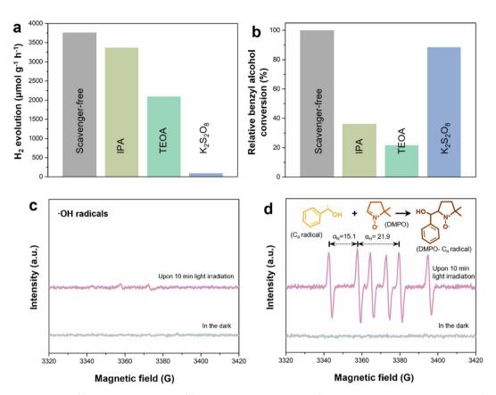
Fig. 6 Scavenger tests for the (a)  $H_2$  evolution rate and (b) benzyl alcohol conversion. Conversion rates are normalized to 100% based on the scavenger-free sample. Condition: scavenger was added same as the mole of benzyl alcohol added. EPR spectra of (c) hydroxyl (\*OH) radicals and (d) carbon-centered (\*CH(OH)Ph) radicals under light irradiation over LZIS-4. The spectra are recorded at 10 min light illumination.
