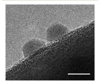
Fig. 7 High resolution TEM image of Pt cocatalyst nanoparticles deposited on a BaTaO<sub>2</sub>N photocatalyst particle. The scale bar is set to 5 nm.
