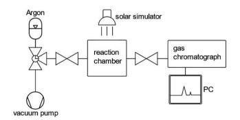
Fig. 2 Schematic representation of an experimental set-up suitable for photocatalytic performance assessment. The gas chromatograph allows the determination of oxygen and hydrogen concentrations in the reaction chamber.
