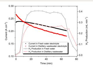
Fig. 6 H<sub>2</sub> generation of Ni<sub>2</sub>Se<sub>3</sub>/SS electrodes using fresh water (black) and distillery wastewater based electrolyte (red). Note that the concentration of electrolytes was 1.0 M NaOH.
