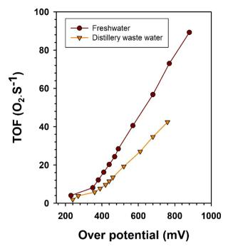
Fig. 7 TOF of Ni<sub>2</sub>Se<sub>3</sub>/SS anode in electrolytic oxygen generation performance in fresh water and distillery wastewater.
