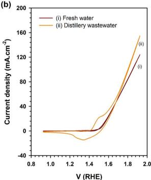
Fig. 3 (a) Linear sweep voltammogram results of stainless steel and Ni<sub>2</sub>Se<sub>3</sub> nanoparticles coated stainless steel substates in freshwater and distillery wastewater electrolyte. (b) CV of Ni<sub>2</sub>Se<sub>3</sub>/SS anode in freshwater and distillery wastewater-based electrolyte. Note that the concentration of the electrolyte was 1 M NaOH.
