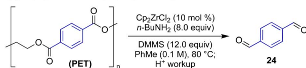
(a) Depolymerization of polyethylene terephthalate from various sources a
