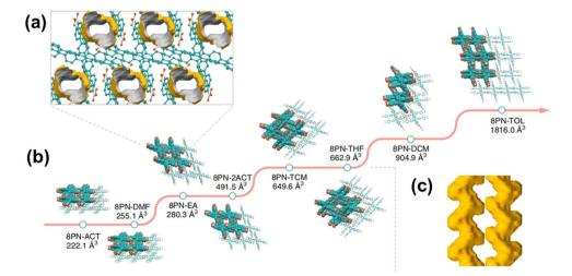
Fig. 14 (a) Packing model of 8PN-EA in the [010] direction, with the solvent-accessible void space; (b) single-crystal X-ray structures of eight 8 PN frameworks with varying void space; (c) S-shaped channel surface of 8PN-THF.<sup>47</sup>
