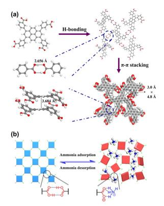
Fig. 8 (a) Crystal structures of FDU-HOF-3; (b) schematic illustration of the self-healing effect of FDU-HOF-3 before and after NH3 capture.64
