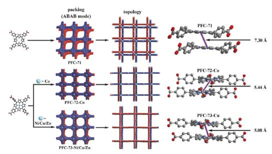
Fig. 19 (left) Schematic representation of the structure and topology of PFC-71, PFC72-Co, and PFC-73-Ni/Cu/Zn; (right) the interlayer porphyrin center-to-center distance of PFC-71, PFC72-Co, and PFC-73-Cu.<sup>61</sup>
