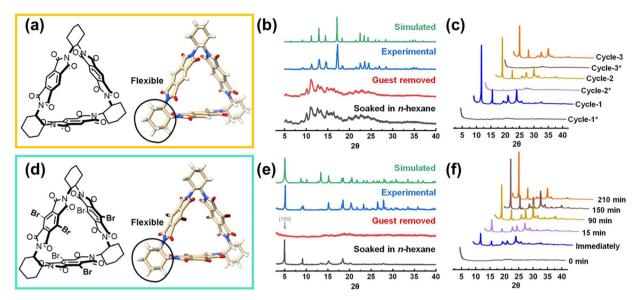
Fig. 10 (a and d) The chemical structures of Tri-PMDI and Tri-PMDI-Br, respectively; (b) PXRD patterns of PMC-Tri-PMDI; (c) PXRD patterns of HOF-Tri-PMDI-Br after removal and resoaking in n-hexane three times; (e) PXRD patterns of HOF-Tri-PMDI-Br; (f) PXRD patterns of HOF-Tri-PMDI-Br soaked in n-hexane for different intervals of time. 62
