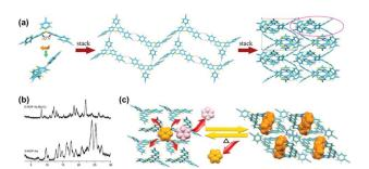
Fig. 15 (a) Assembling of PTTCN molecules (left) to a 2D H-bonded framework with pores (middle), and intermolecular stacking in a 2  $\times$  2 cell (right); (b) PXRD patterns; (c) schematic representation of the separation for benzene/cyclohexane.<sup>93</sup>
