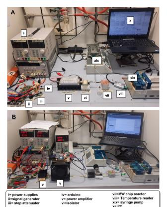
Fig. 3 A) Complete setup working up to 2.5 GHz. B) Complete setup working between 6-12 GHz.
