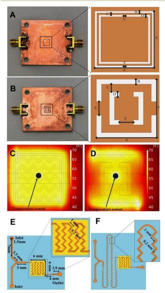
Fig. 1 A) 2 GHz CSRR. B) 8 GHz CSRR. C) COMSOL MW heating simulation with input power of 1 W at 2 GHz. D) COMSOL MW heating simulation with input power of 1 W at 8 GHz. E) Flow cell A. F) Flow
