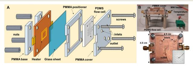
Fig. 2 A) Schematic representation of the μw-μf-CR. B) Picture of the assembled μw-μf-CR seen from the side (top image) and the top (bottom image).
