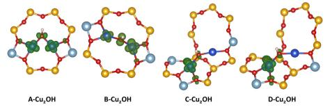
Fig. 5 LUMO orbitals of Cu<sub>2</sub>OH sites in different dimer anchoring configurations. The LUMO charge isosurfaces are shown in green, Cu atoms in blue, Si atoms in yellow, O atoms in red, H atoms in white, and Al atoms in grey.
