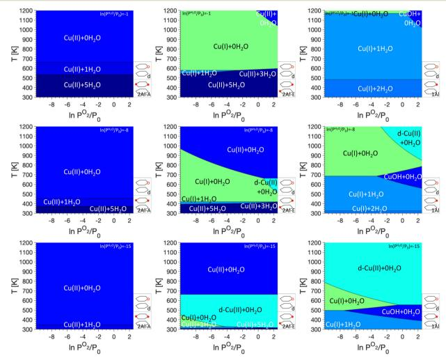
Fig. 3  $P^{O_2}/T$  phase diagrams for monomers anchored in 2Al-A (left), 2Al-E (middle), and 1Al with defects included at different  $P^{H_2O}$  values. Regions of uniform color correspond to the site indicated by the label. Schematics of the included anchoring configurations are shown in the bottom right and PH2O values are given in the legend on the top right.
