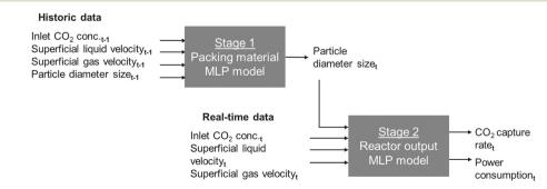
Fig. 2 The two-stage multilayer perceptron network (MLP) dynamic model to predict CO2 capture rate and the power consumption of the enhanced weathering packed bubble column reactor with respect to deteriorating packing material size.
