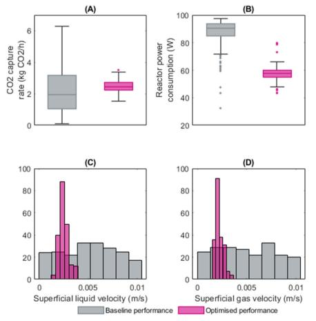
Fig. 6 Comparing baseline and optimised performance of the enhanced weather reactors for the (A) CO<sub>2</sub> capture rate and (B) reactor power consumption, including the optimised operating conditions (C) superficial liquid velocity and (D) superficial gas velocity.
