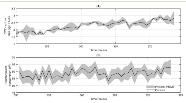
Fig. 7 Comparison of CO<sub>2</sub> capture rate (A) and reactor power consumption (B) predictions against actual values, including prediction intervals determined using conformal prediction, over a 24 hour operation of the reactors using unseen data.
