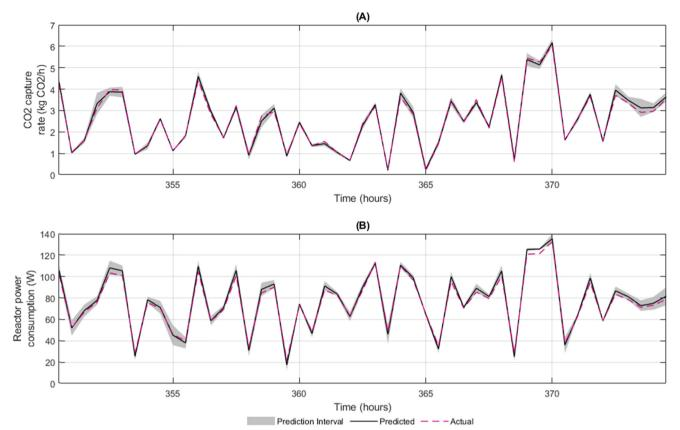
Fig. 4 Comparison of CO2 capture rate (A) and reactor power consumption (B) predictions against actual values, including prediction intervals determined using conformal prediction, over a 24-hour operation of the reactors using unseen data.
