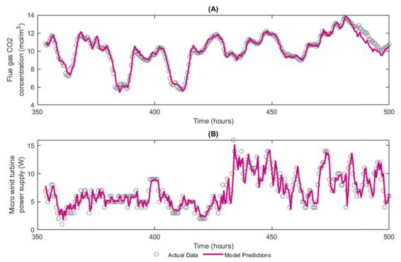
Fig. 5 Comparison between the actual (A) CO<sub>2</sub> concentration in flue gas and (B) the power output from the micro wind turbine against the corresponding LSTM model predictions for the testing data. The solid line represents the model's predictions, while the scattered data points indicate the actual data.
