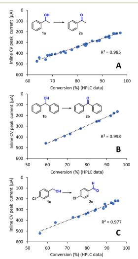
Fig. 5 Comparison of the inline CV response with offline HPLC conversion data for the preparative-scale oxidation of (A) 1a, (B) 1b and (C) 1c. The setup shown in Fig. 4 was used in all cases. The  $R^2$  for linear regression is also shown.
