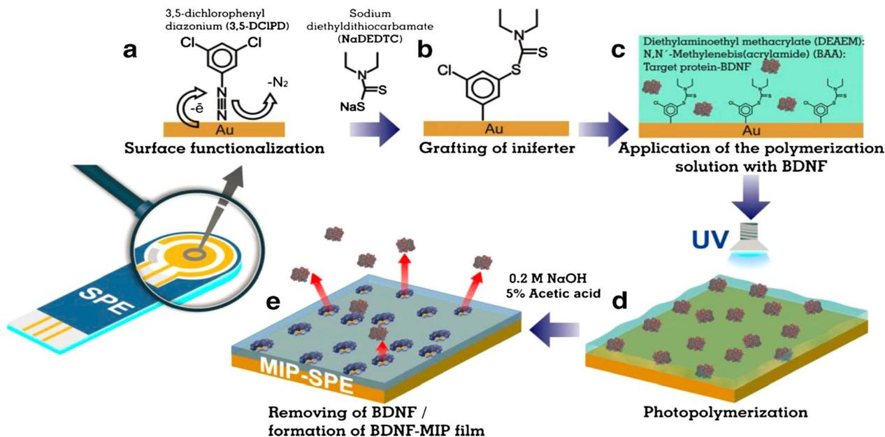
Fig. 1 Schematic of the steps involved in surface-initiated polymerization.<sup>52</sup>
