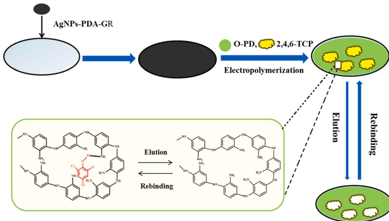
Fig. 16 MIP/AgNP-PDA-GR/GCE fabrication.<sup>87</sup>
