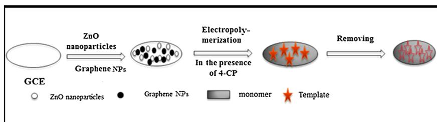
Fig. 6 Fabrication of the GCE/ZnO/GNPs/MIP.<sup>72</sup>
