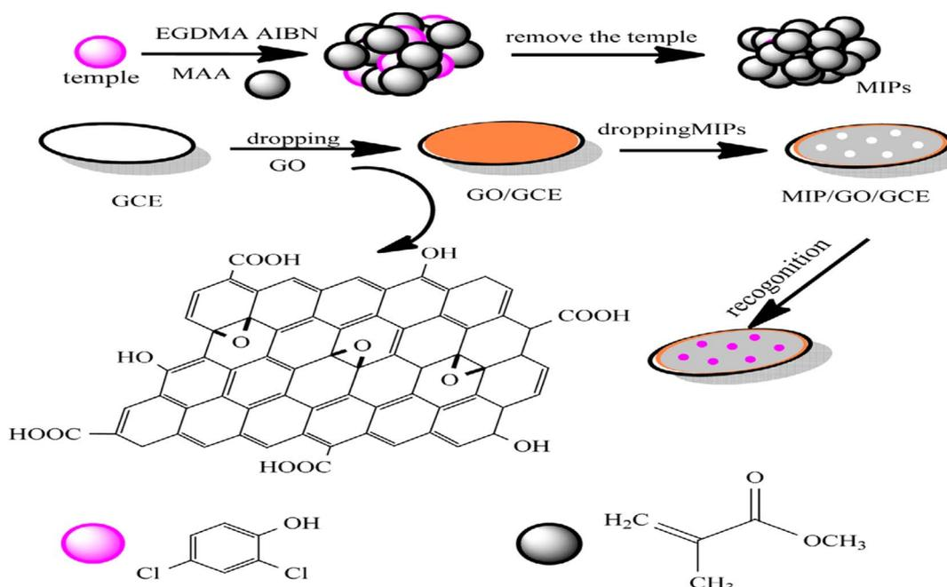
Fig. 11 Construction of the improved electrode and synthesis of the molecularly imprinted polymer.<sup>75</sup>
