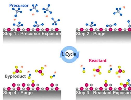
Fig. 3 Schematic diagram of thin layer formation process in ALD<sup>99</sup> (Copyright (2009) Elsevier).
