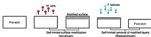
Fig. 4 Schematic view of a single silicon nitride quasi-ALE cycle<sup>103</sup> (Copyright (2017) AIP publishing).
