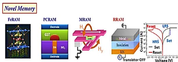
Fig. 15 Non-volatile memory devices, such as MRAM, PCRAM, and FeRAM<sup>168</sup> (Copyright (2016) *Materials Today*).
