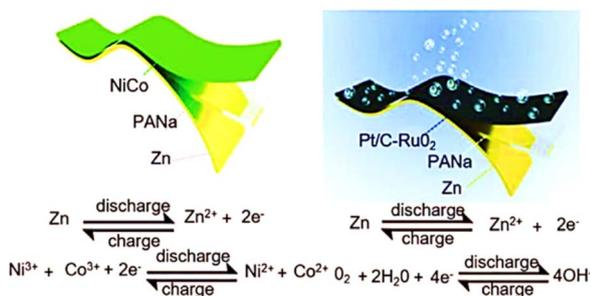
Fig. 16 Zn anode, NiCoOH cathode, and PANA polyelectrolyte composed the Zn//NiCo battery<sup>180</sup> (Copyright (2018) *Advanced Energy Materials*).
