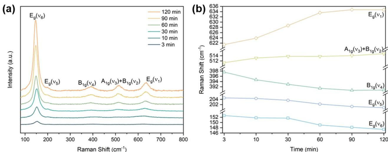
Fig. 4 (a) Raman spectrum of TNTAs grown for 2 h and annealing at 300 °C, (b) peak positions of the five Raman peaks of anatase phase at 300 °C annealing versus annealing time.
