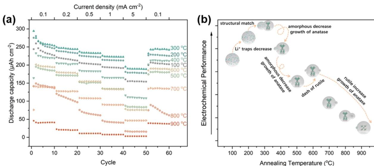
Fig. 7 (a) High rate cycling performance of TNTAs grown for 2 h and annealing at different temperatures. Current density is 0.1–5  $\text{mA cm}^{-2}$ . (b) Relationship between electrochemical properties and annealing temperature.
