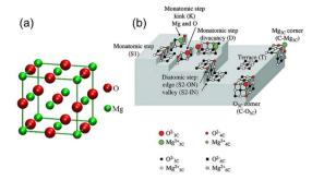
Fig. 3 (a) Crystal structure of MgO.<sup>34</sup> Reprinted with permission from ref. 34. Copyright © 2010, IOP. (b) Schematic representation of irregularities on the surface of MgO. The terminologies used are shown in Table 2.  ${\rm M_{3c}}^{2+}$ : 3-coordinated  ${\rm Mg}^{2+}$  on corners;  ${\rm O_{4c}}^{2-}$ : 4-coordinated  ${\rm O}^{2-}$  on edges.<sup>35</sup> Reprinted with permission from ref. 35. Copyright © 2011, Taylor & Francis.
