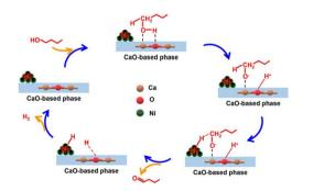
Fig. 9 Synergistic catalysis reaction mechanism via the metal and base sites for the dehydrogenation of n-butanol.<sup>76</sup> Reprinted with permission from ref. 76. Copyright © 2020, the American Chemical Society.
