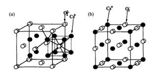
Fig. 13 Bonding structures of various cesium oxides. (a)  $Cs_2O_2$  and (b)  $Cs_2O_4$ . <sup>122</sup> Reprinted with permission from ref. 122. Copyright © 1997, Elsevier.
