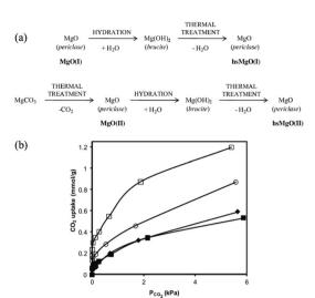
Fig. 2 (a) Proposed activation steps and notation (bold) used for the different MgO. (b)  $CO_2$  adsorption isotherms at 50 °C and 6.7 kPa, measured by microcalorimetry for MgO(I) ( $\spadesuit$ ), MgO(II) ( $\blacksquare$ ), hs MgO(I) ( $\square$ ), and hs MgO(II) ( $\bigcirc$ ). Reprinted with permission from ref. 31. Copyright © 2014, Elsevier.
