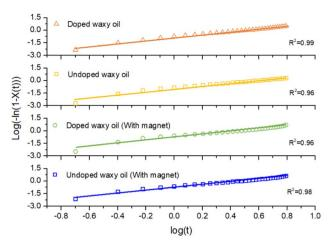
Fig. 10 Avrami fitting diagram for the waxy oil under magnetic treatment.
