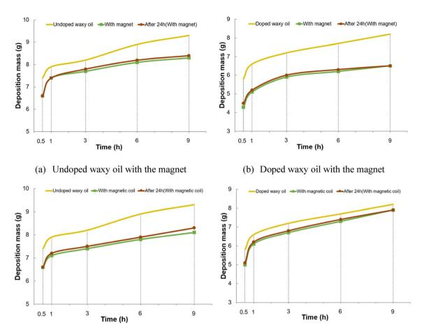
Fig. 2 Wax deposition process after magnetic treatment with 0 and 24 h of resting.
