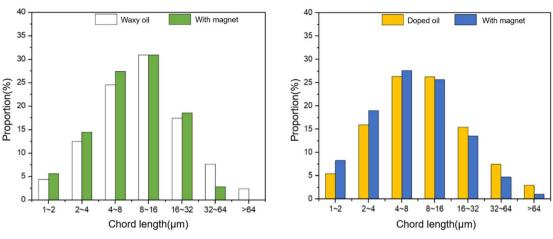
(a) Size distribution of wax crystals in the undoped waxy oil before and after magnetic treatment
