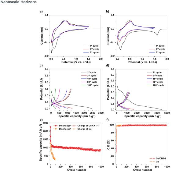
Fig. 4 Cyclic voltammetry diagrams of (a) Ge electrode and (b) Ge/CNT-1 electrode. Discharge—charge profiles of (c) Ge electrode and (d) Ge/CNT-1 electrode. (e) Cyclability with (f) coulombic efficiency of Ge electrode and Ge/CNT-1 electrode at C/5.
