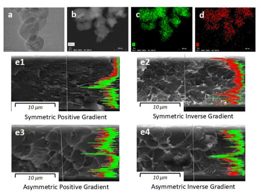
Fig. 2 The TEM image (a) and elemental mappings (b)-(d) of the BNNSs. (e) The cross-sectional SEM images and elemental mappings of the gradient composite dielectrics
