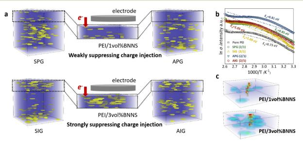
Fig. 5 (a) Schematic diagram of the metal/dielectric interface. (b) Dependence of  $\ln \sigma$  on 1000/T for the pure PEI, SPG (2/1), SIG (2/1), APG (2/1), and AIG (2/1) composite dielectrics at  $10^2$  Hz. (c) Development of the breakdown path in the surface barrier layer.
