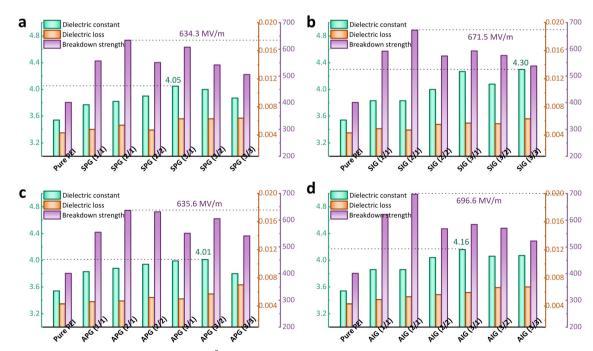
Fig. 3 The dielectric constant and dielectric loss at 10<sup>2</sup> Hz, as well as the breakdown strength of (a) SPG, (b) SIG, (c) APG, and (d) AIG composite dielectrics
