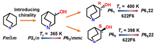
Fig. 11 Scheme representing the introduction of homochirality in 3-quinuclidinol. Reprinted (used in part) with permission from ref. 118. Copyright 2020 American Chemical Society.
