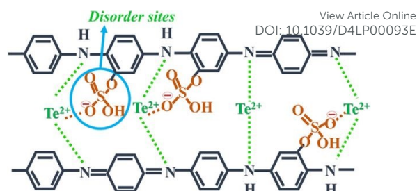
Figure 5. Charge transport mechanism in Te-PANI [Reproduced from ref. 34, with permission from Springer Nature, copyright 2023]
