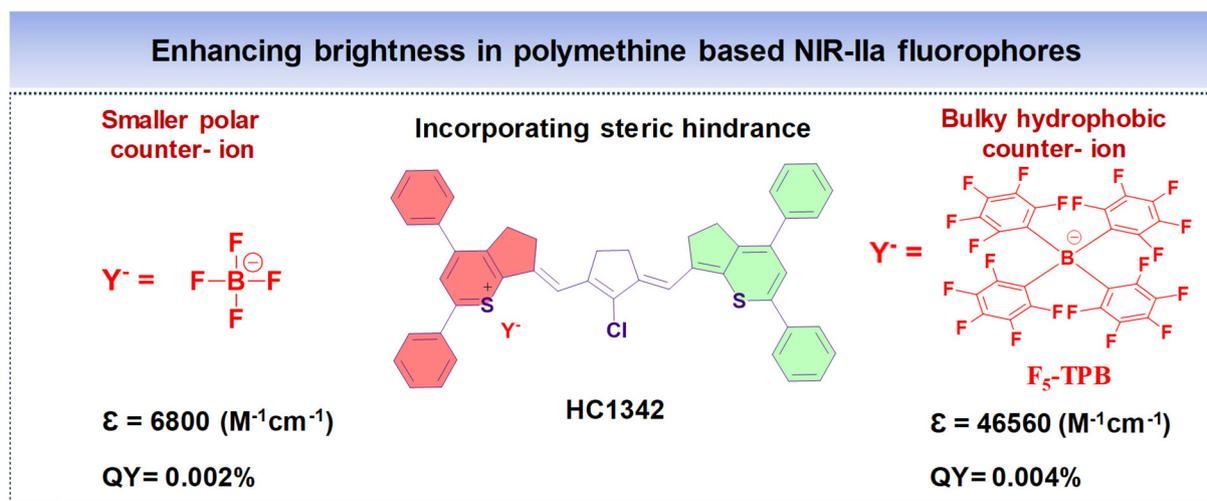
**Fig. 12** Enhancing the NIR-IIa brightness of polymethine based fluorophore HC1342 by introducing steric hindrance from smaller and bulky counter-ions.
