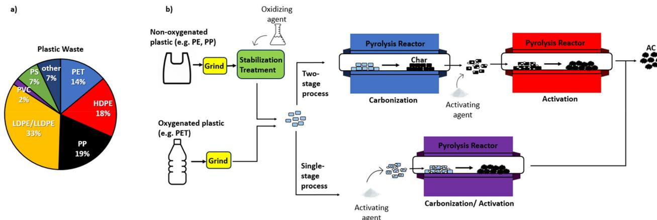
**Fig. 6** (a) Composition of plastic waste managed in the US in 2019. Data obtained from ref. 11; (b) illustration of various pathways for the chemical activation of oxygenated and non-oxygenated plastics.
