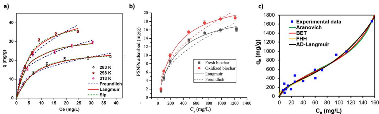
**Fig. 10** Adsorption isotherm curves of (a) PS NPs onto sugarcane Bagasse biochar at varying adsorption temperatures. Adapted from ref. 200 with permission from Elsevier. Copyright ©2021; (b) PS NPs onto oxidized and non-oxidized corncob biochar. Adapted from ref. 201 with permission from Elsevier. Copyright ©2021; and (c) PET NPs onto epoxy AC. Adapted from ref. 110 with permission from Elsevier. Copyright ©2023.
