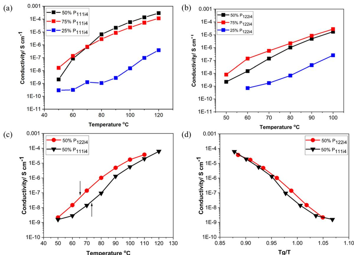
**Fig. 2** Ionic conductivity at different concentrations of poly-NaMTFSI with (a) poly- $P_{111i4}$ MTFSI and (b) poly- $P_{122i4}$ MTFSI, (c) ionic conductivity of 50 mol% polymer blends of the mixed co-cation of poly- $P_{111i4}$  and poly- $P_{122i4}$  with poly-NaMTFSI. (d) Ionic conductivity as a function of the bulky cation with inverse temperature normalized by  $T_g$  for each polymer blend.
