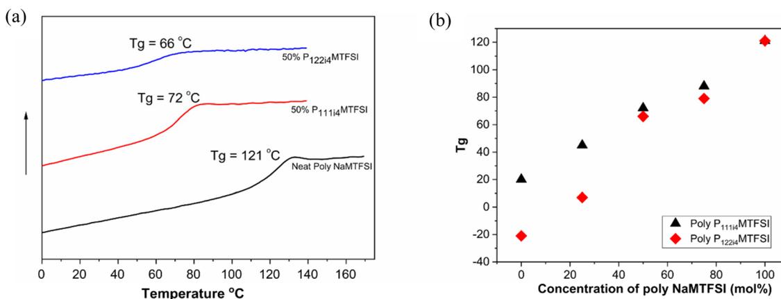
**Fig. 1** (a) DSC thermograms of neat poly-NaMTFSI and 50 mol% poly-P<sub>11114</sub>MTFSI and poly-P<sub>12214</sub>MTFSI polymer blends. (b)  $T_g$  of different polymer blends with poly-NaMTFSI with both poly-P<sub>11114</sub>MTFSI and P<sub>12214</sub>MTFSI at different compositions. Scan rate: 10 K min<sup>-1</sup>.
