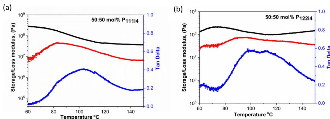
Fig. 3 Storage modulus ( $E'$ , black), loss modulus ( $E''$ , red) and  $\tan \delta$  (blue) as a function of temperature for the 50 mol% polymer blends of the mixed co-cation of poly-NaMTFSI with (a)  $P_{111i4}$ MTFSI and (b)  $P_{122i4}$ MTFSI.
