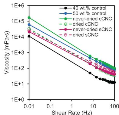
**Fig. 2** Viscosity as a function of angular frequency of BA/MMA liquid latexes containing CNCs with different surface functionalities (carboxylated vs. sulfated) and storage methods (never-dried vs. dried).
