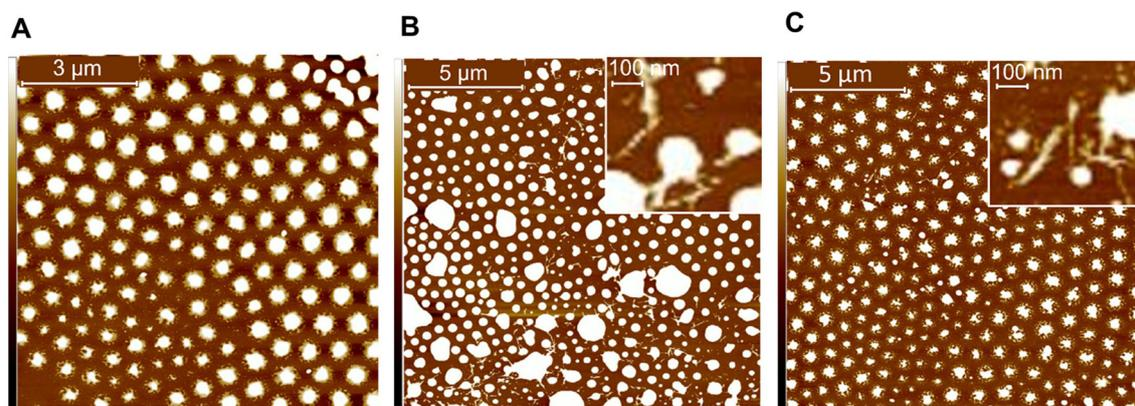
Fig. 3 AFM height images of BA/MMA latex films with (A) 40 wt% control (no CNCs), (B) 1 wt% dried cCNCs and (C) 1 wt% dried sCNCs. Image has a height scale from –10 to 10 nm.
