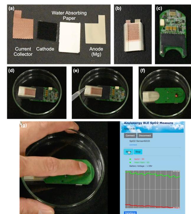
**Fig. 4** Photographs of cell components (a), a single paper battery cell (b),  $\text{SpO}_2$  sensor (c),  $\text{SpO}_2$  sensor with the cell (d), injection of salt water to the cell (e), and the active  $\text{SpO}_2$  sensor (other side compared with panels (d) and (e)) (f). Real-time monitoring of  $\text{O}_2$  saturation and pulse measured in a person (g).
