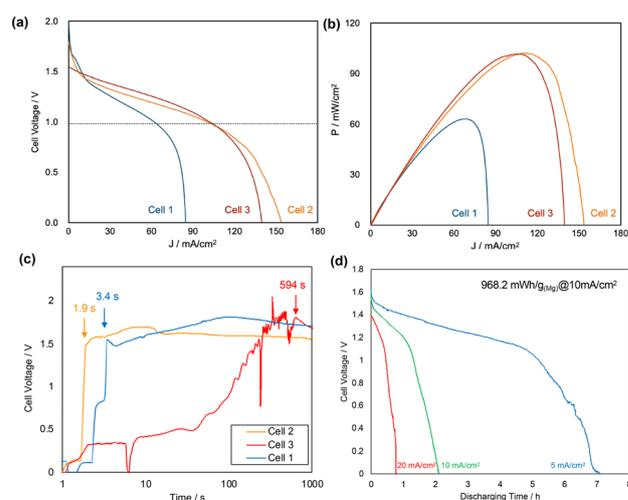
Fig. 2 *I*-*V* (a) and *I*-*P* (b) polarization curves of the cells (cell 1 (blue), cell 2 (yellow), and cell 3 (red)), time dependence of cell voltages of the cells after water activation (c), and discharge polarization curves of cell 2 at 5 (blue), 10 (green), and 20 mA cm<sup>-2</sup> (red) (d).
