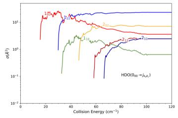
Fig. 12 Cross sections for the excitation of the fundamental  $0_{00}$  rotational level of the HOD molecule by collision with *normal*-H<sub>2</sub>. The curves on the log-linear plot correspond to transitions to the first six rotational excited states.
