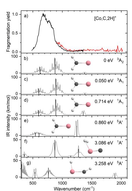
Fig. 4 (a) Experimental IRMPD spectrum of [Co,C,2H]<sup>+</sup>, the black trace is the average of two scans, the red trace is a single scan; (b)–(g) B3LYP/def2-TZVPPD calculated IR spectra of different [Co,C,2H]<sup>+</sup> states and isomers with the harmonic vibrations in black and the rovibrational envelopes in grey accompanied by geometric structure, relative energy, and electronic state.
