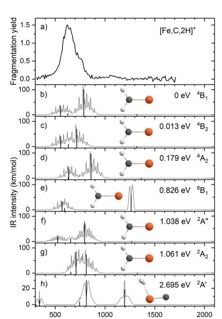
Fig. 1 (a) Experimental IRMPD spectrum of [Fe,C,2H]<sup>+</sup>; (b)–(h) B3LYP/def2-TZVPPD calculated IR spectra of different [Fe,C,2H]<sup>+</sup> states and isomers with the harmonic vibrations in black and the rovibrational envelopes in grey accompanied by geometric structure, relative energy, and electronic state.
