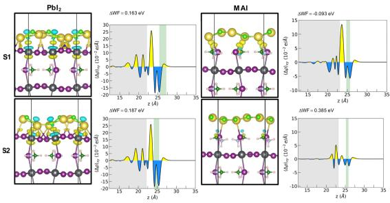
Fig. 3 Electron density differences for the interaction between the Pbl2- and the MAI-terminated MAPI film and the NaCl layer (left). Yellow denotes increased electronic density and light blue indicates decreased electronic density. Isosurface value: 0.0025. Planar average charge density difference for each system (right). Color code: Pb - dark gray; I - violet; C - green; N - light blue; H - light pink; Na - yellow; Cl - light green.
