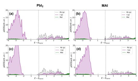
Fig. 4 Projected density of states (pDOS) calculated at the PBE level of theory for the S1 configuration of both surface terminations. Upper plots (a) and (b) refer only to the perovskite with an iodine vacancy. In pictures (c) and (d), the same analysis is shown for the same systems with the salt coverage.
