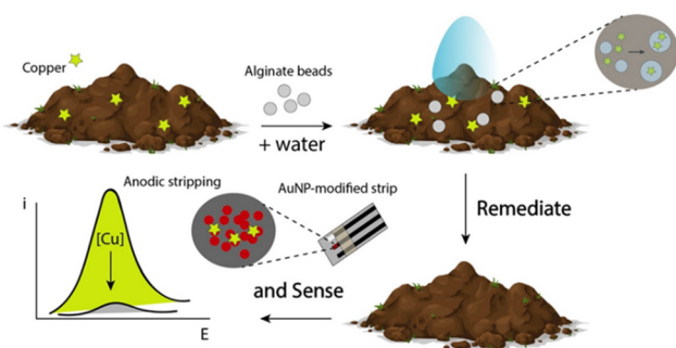
Fig. 1 Architecture mechanism of the remediate-and-sense concept carried out in soil samples.
