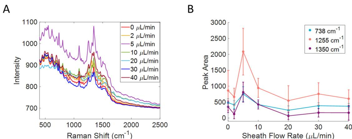
**Fig. 2** Optimizing flow parameters for molecule detection in 3D printed flow cell using riboflavin as a model analyte. Raw spectra at varying sheath flow rates is shown in (A), while the sample flow rate was kept constant at  $1 \mu\text{L min}^{-1}$ . 3 peaks arising from riboflavin were fit and the corresponding peak area was plotted against sheath flow rate (B). The signal was most intense when a sheath flow rate of  $5 \mu\text{L min}^{-1}$  was used.
