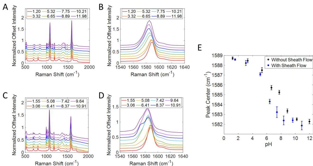
**Fig. 3** SERS spectra of MBA while flowing PBS solutions over the surface at varying pH values with sheath flow off (A) with a zoom in on the  $1585 \text{ cm}^{-1}$  band (B), and with sheath flow on (C & D). The center of the  $1585 \text{ cm}^{-1}$  band was used to create a titration curve (E). The inflection point on this curve is much sharper when the sheath flow was on.
