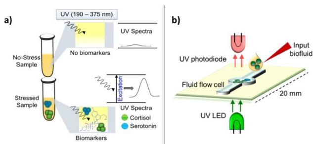
**Fig. 4** Optical absorption approach for label-free biomarker detection: (a) basic absorption function; (b) integration approach. Reproduced from ref. 70 with permission from American Chemical Society, copyright 2019.
