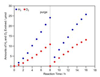
Fig. 6 Time course of water-splitting activity for the Pt<sub>NC</sub>/STO:Rh-BiVO<sub>4</sub> composite Z-scheme system using FeCl<sub>2</sub> as a mediator. Light source: a 300 W Xe lamp with a long-pass filter (>  $\sim$  410 nm), catalyst: 100 mg for each catalyst, reactant solution: 120 mL of 2 mmol  $L^{-1}$  FeCl<sub>2</sub> in  $H_2SO_4$  aq. (pH 2.4), reaction cell: a top-window reaction cell.
