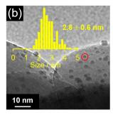
Fig. 3 TEM images and resulting histograms (inset) for the particle-size distribution of Pt cocatalysts in (a) Pt<sub>NC</sub>/STO:Rh and (b) Pt<sub>PD</sub>/STO:Rh.
